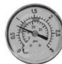
0,8 kg/cm 2 - 11,4 PSI: Normal pressure at the beginning of a filtering cycle.
